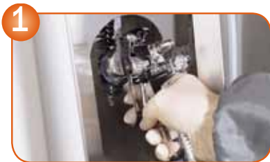
Clean and rinse material passage and air cap
