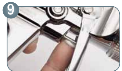
Grease visible part of air piston rod
