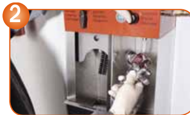
Blow dry spray gun and material passage
