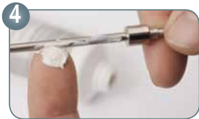
Grease paint needle around the needle packing area
