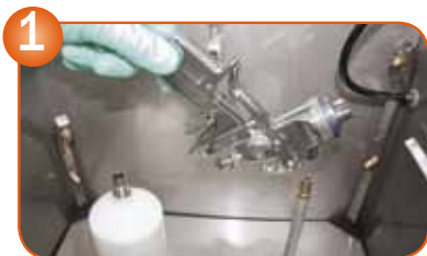
Ensure correct position of spray gun
