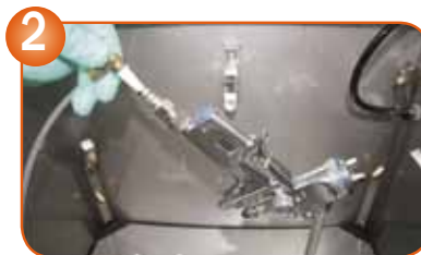
Connect air connection to air inlet
